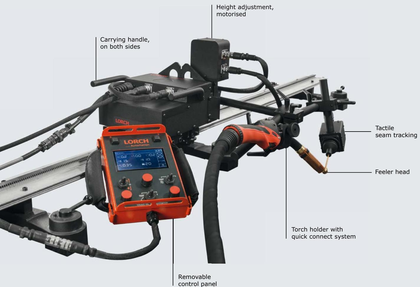
Fig. Without power supply unit
