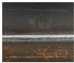
The detailed view also shows how even the weld seam performed by the tractor is.
