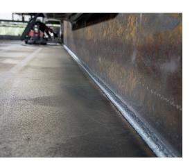
The tractor advantage for a perfect weld seam from start to finish. The optimal weld setting prevents spatter and eliminates time-consuming rework.
