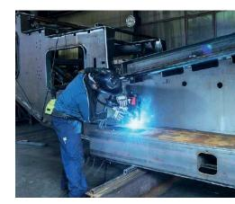
Set up the unit, adjust the values, and start welding. A magnet allows easy fastening of the tractor, while a high-performance motor ensures a precise welding speed.
